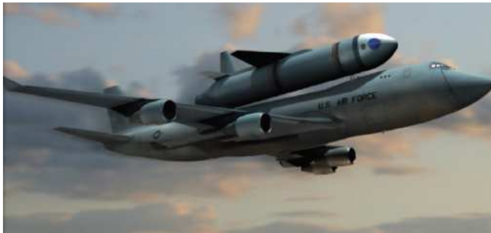
Figure I. Conceptual image of air launch method from a B747-400 aircraft. Courtesy of NASA, 2011, HLS-SP 2011-215994, p. 30.
